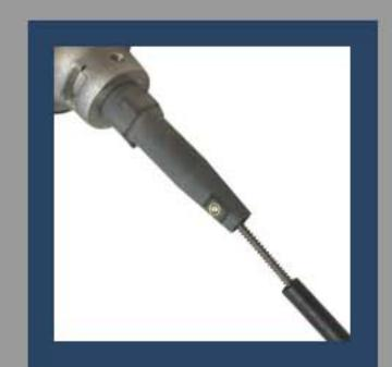
Slide the outer sheath onto the cable until it reaches the motor.
