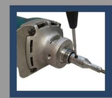
Secure the inner cable to the motor using the set screw on the cable.
